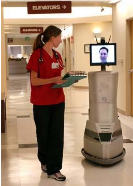
A "rounding robot" rolls down a corridor at Mission Hospital in Mission Viejo, Calif., with Dr. Thomas Shaver's face displayed on a video screen. The contraption lets the physician interact with patients from a remote location.
