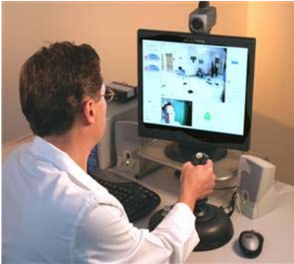
Dr. Thomas Shaver, a surgeon at Mission Hospital in Mission Viejo, Calif., operates InTouch Health's robot remotely using a joystick. Shaver sees what's going on via a video link, and a Webcam focused on his face helps him interact with patients.
